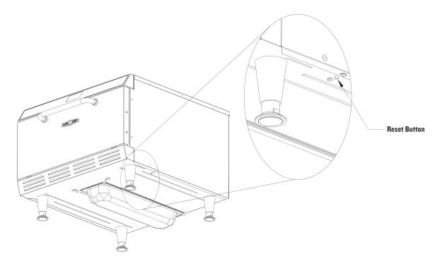
FIGURE 25: Location of Hi-Limit Thermostat Reset Button
